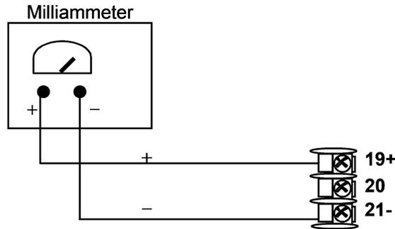
Table 7-1: Set Up Wiring Procedure for Current Output
