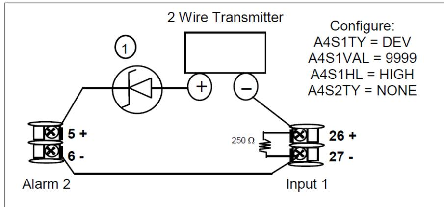
Figure 3-17: Transmitter Power for 4-20 mA – 2 Wire Transmitter Using Auxiliary Output
