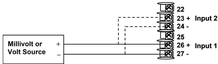
Table 6-5: Set Up Wiring Procedure for Millivolts, Volts or Thermocouple Differential Inputs
